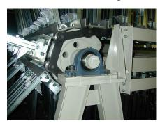
the industry, featuring oversize frame rails and runways, massive 3" diameter front and rear shafts (large-diameter shafts resist twisting when the Carrier is being indexed from section to section by the drive motor; 3" shafts are 4 times stiffer and stronger than 2" diameter shafts). big cast iron sprockets, heavyduty chains with 2" wide rollers, and extra-stout 6" I-beam legs. Machines are available to handle stock up to 20.5' long and 8" thick. Frames are expandable to up to 80 sections.
