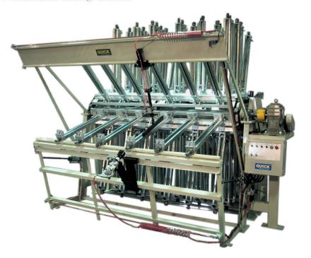
Heavy Duty 20-section Hydraulic Clamp Carrier
