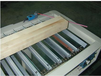
Mounted on the motor shaft is an adjustable slip clutch, which helps ensure operator safety, and helps prevent crossbars from bending should material inadvertently get jammed in the conveyor.
