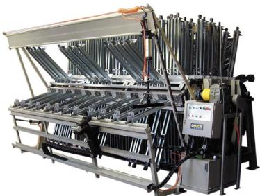
Our Heavy-Duty Clamp Carriers are designed for high production and super durability. The frames (and clamps) on these machines are the heaviest and stiffest in the industry, with oversize frame rails and runways, 3" diameter front and rear shafts, heavy-duty chains with 2" wide rollers, large cast iron sprockets, and massive 6" I-beam legs. Pneumatic and Hydraulic Clamp Tighteners are available. Machine widths are available from 6.5' to 16.5'. From 6 to 80 sections, expandable.
