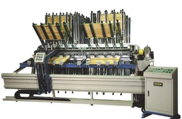
Our Automatic Clamp Carrier brings full automation to the panel clamping process. After loading the clamps with stock, the operator simply presses the "Cycle Start" button, which commences the machine's fully automatic clamp tightening, Carrier rotation, clamp loosening cycle.
