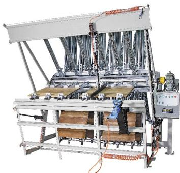
Our Standard Clamp Carriers are our mid-size gluing machines. Providing the best bang-for-the-buck in the industry, they include zinc-plated, full box-frame clamps, super-fast 3000 RPM Pneumatic Clamp Tighteners, Pneumatic Panel Flatteners and Electric Motor Drives with Automatic Rotation Cycles. Standard width is 8.5'; standard clamp opening is 38"; other sizes are available. Available with 6, 14 or 20 sections. Expandable later to 14 or 20 sections.
