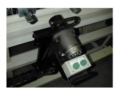
Our High Production Clamp Carrier frames are the heaviest, strongest and stiffest in the industry. 20-section and larger frames have oversize frame rails and runways, massive 3" diameter front and rear shafts (large-diameter shafts resist twisting when the Clamp Carrier is being indexed from section to section by the drive motor), big cast iron sprockets, heavy-duty chains with 2" wide rollers, and extra-stout 6" I-beam legs.
